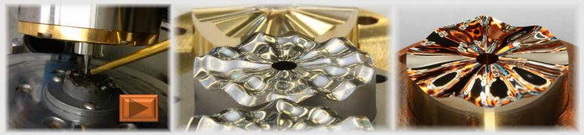
Flat nickel mirror milling results – machined with an ASD080C6 on a Precitech machine
