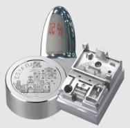
**Reflectors made from steel & brass** – milled at Levicron with an ASD080C6 (click for machining video)
