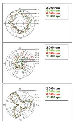
To verify our spindles' quality and precision, Levicron has developed its error-motion testing rig, data acquisition, and software.
